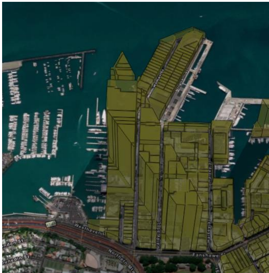
Figure 3: Example of height split in Wynyard Quarter displaying more than one height in a parcel.
